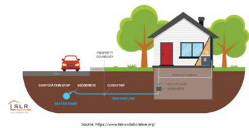
Figure 1. Example Lead Service Line Schematic Source: https://www.lslr-collaborative.org/
