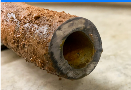
Harvested lead service line
